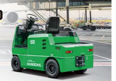
The wide-view cab with an integral frame is flexibly connected to the body, and has good sealing, sound insulation, vibration isolation and heat insulation, etc. as well as a large operation space to improve the driver's comfort.
